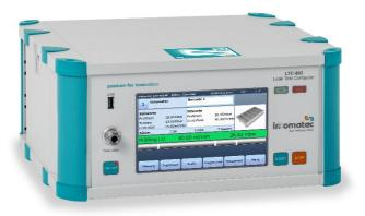
The LTC-802 M-Performance offers a high-precision leak testing solution based on the mass flow method in a compact package that can be implemented without a reference volume. The improved design allows for shorter cycle times and reduces the time required to calibrate components.
